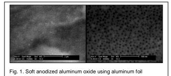
The SEM micrograph shown in Figure 1 is the surface of the substrate after soft anodization of aluminum foil. It is visible in here that the pores are regular and the diameters of these pores are about 40 to 60 nm.
