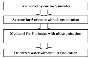
These steps are necessary in order to prepare the surface of metal for a better quality anodized aluminum oxide.
