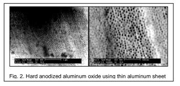
Figure 2 shows the regular pattern after hard anodization of thin aluminum sheet. The pore diameter produced in this two step anodization process is around 50 to 70 nm. Evident from this micrograph is the uneven surface of the aluminum metal surface prior to anodization.
